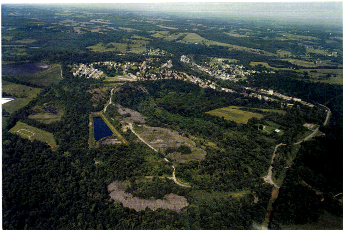
Figure 17. Spoil piles from traditional room-and-pillar mining at Marianna, Washington County. Small wetlands in the vicinity are not visible from the air or identified by the National Wetland Inventory.
